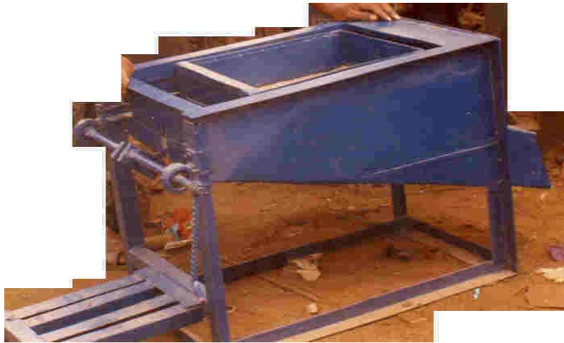
Fig. 1. The gari sifter with handle for manual operation
