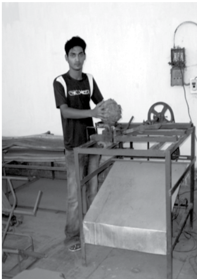
Fig. 2: Working of power operated coconut dehusker
