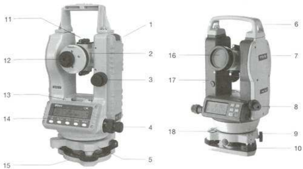
Figure 3.3 – Nikon NE100 and Pentax PTH-10 electronic theodolites: 1 battery compartment; 2 telescope focus; 3 vertical clamp and tangent screw; 4 horizontal clamp and tangent screw; 5 tribrach; 6 carrying handle; 7 vertical circle; 8 optical plummet; 9 tribrach clamp; 10 footscrew; 11 collimator (sight); 12 eyepiece; 13 plate level; 14 keyboard and display; 15 trivet; 16 objective; 17 standard; 18 circular bubble (courtesy Survey Supplies and Pentax UK Ltd).
