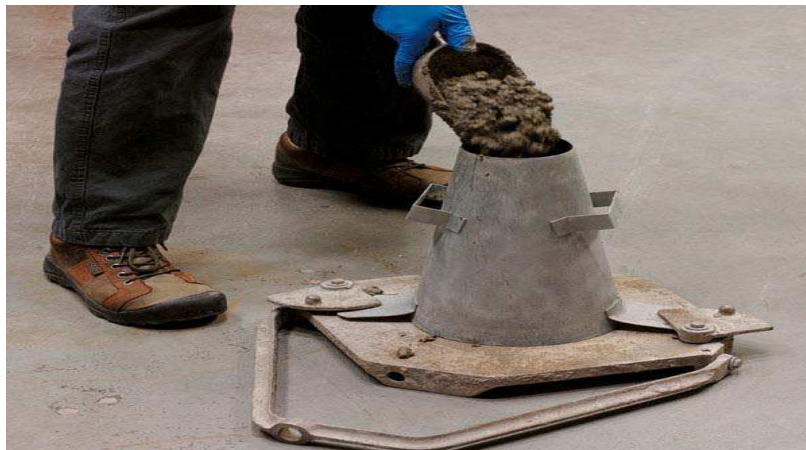
Filling the slump cone
