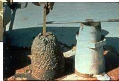
20 Levelling, removing cone and measuring
