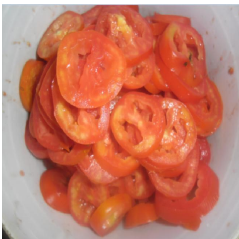
Plate I: 5mm Sliced and Deseeded Fresh Tomato Sample used for the Drying Experiment
