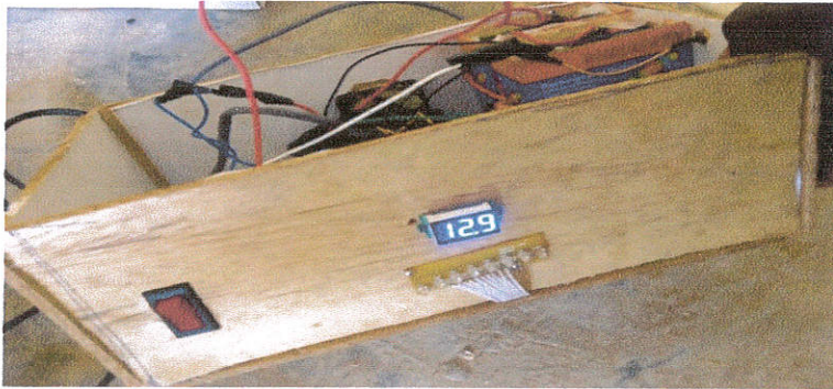
Fig. 12 Interconnection with the LCD
