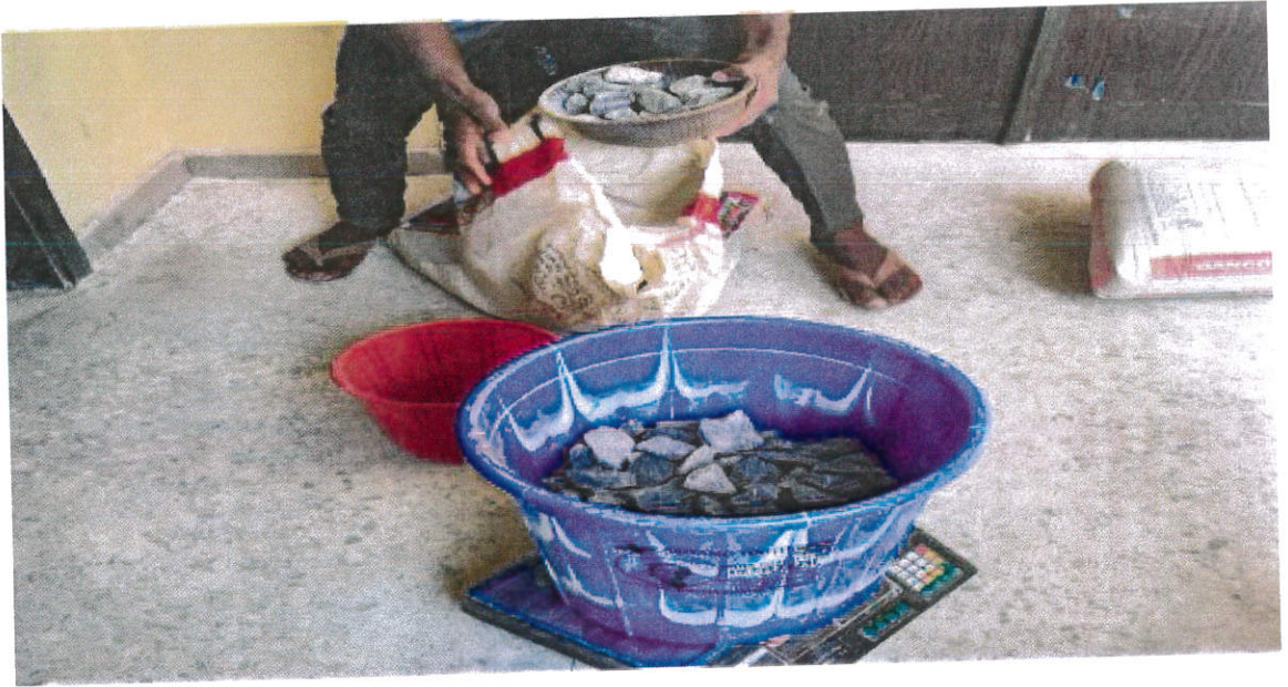
Plate 3.3 Weighing of the materials for casting
