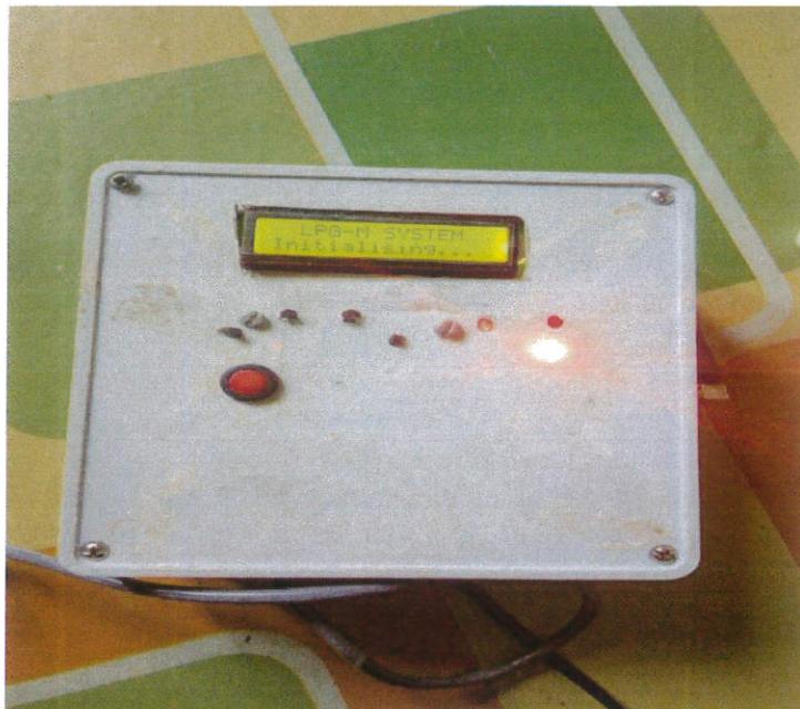
Figure 4.2: Development Board after Component Implementation
