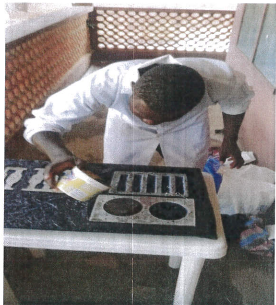
Plate 7: Pouring of Composites inside mold
