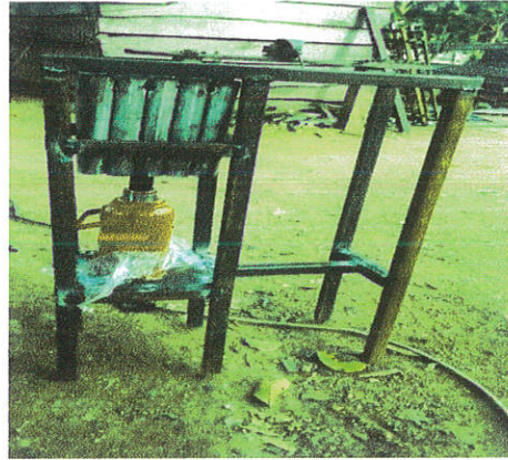
Plate3.4: Frame and mould box after construction
