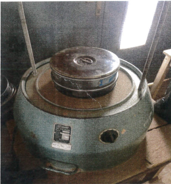
Plate 3: Seive Analysis of Groundnut Shell Particle
