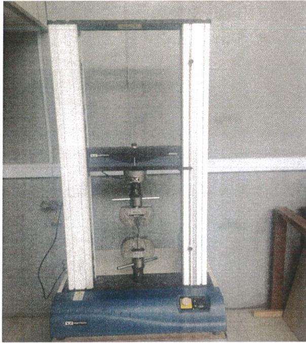
Plate 10: Double cell Universal instron machine (Instron 3369)
