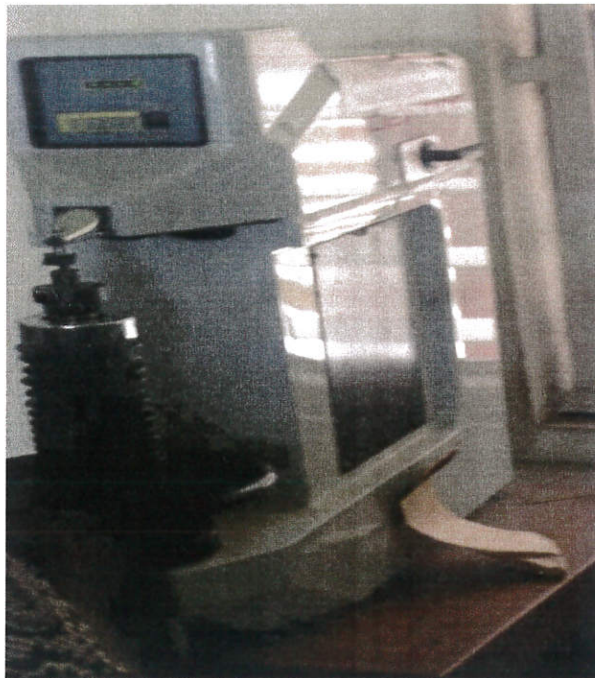
Plate 11: An Electric powered Rockwell hardness testing machine (HRA 60)
