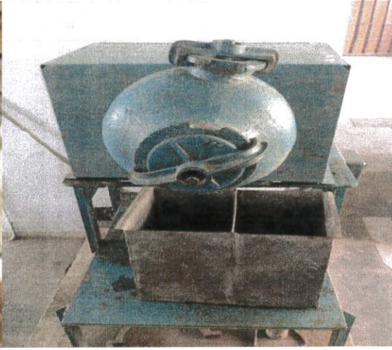
Plate 2: Crushing and Grinding of Groundnut shell
