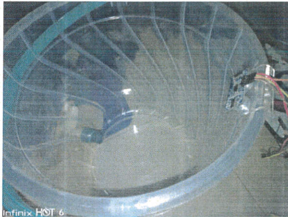
Figure 11: Picture of the mini water tank and the positioning of the ultrasonic sensor
