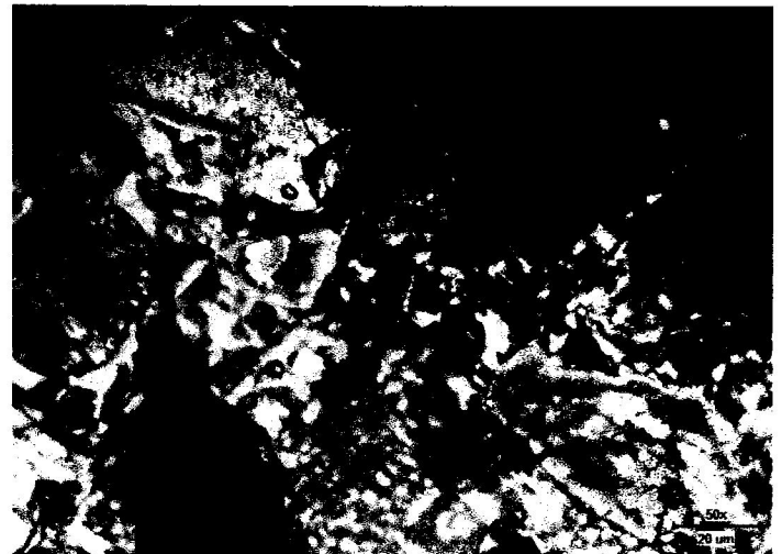
Plate 4.6: Photomicrograph of Lokoja sandstone FE2A under XPL (Mg X50) (MQ - Monocline Quartz, MF - Microcline Feldspar, B- Biotite) (Long. 06^{\circ} 042' 43'' , Lat. 07^{\circ} 51' 15.0'' )
