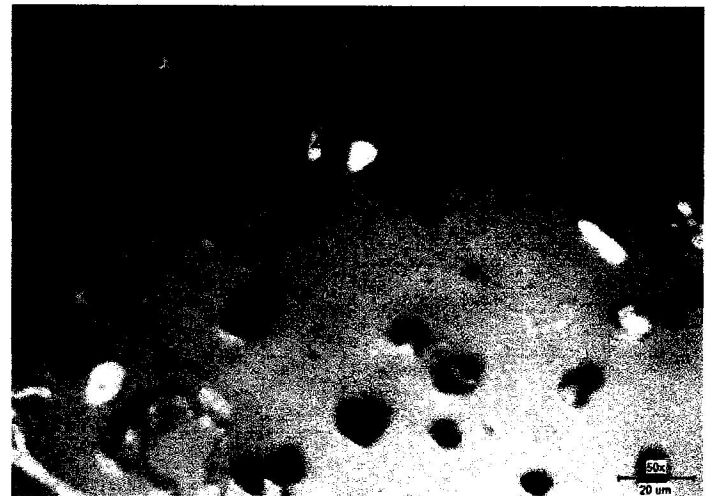
Plate 4.12: Photomicrograph of heavy minerals in Lokoja sandstone (FE1C) showing Zircon (Z), Opaque Minerals (Op), Tourmaline (Tr), Rutile (R) under XPL (Long. 07^{\circ} 51' 18'' E, Lat. 006^{\circ} 41' 54.5'' N)
