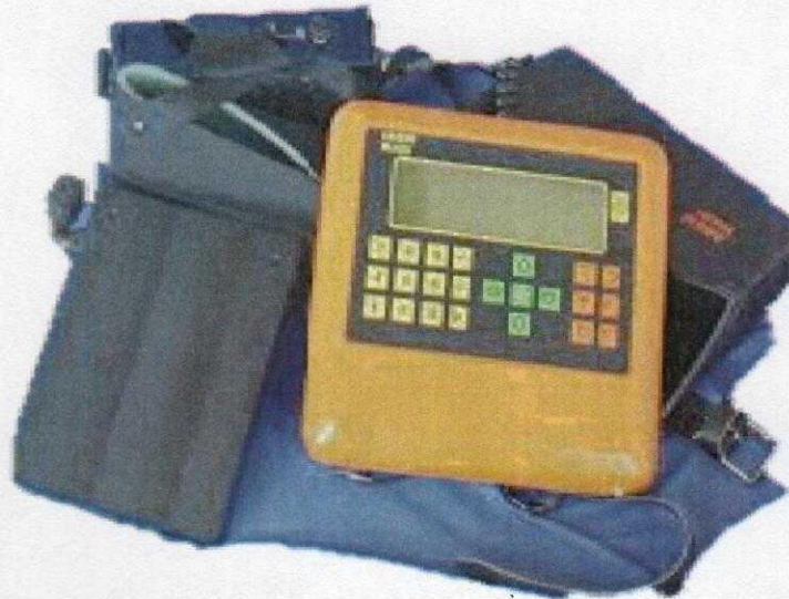
Figure 3.1: ABEM-WADI VLF-EM Equipment
