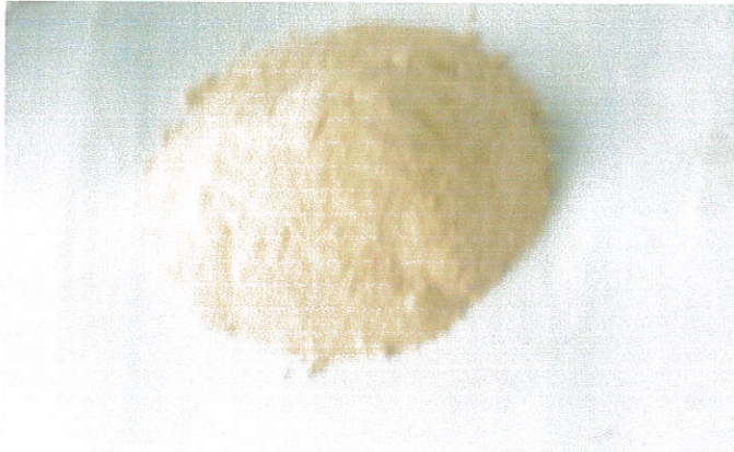
Figure 3.1: (b) Snail Shells after grinding using ball mill
