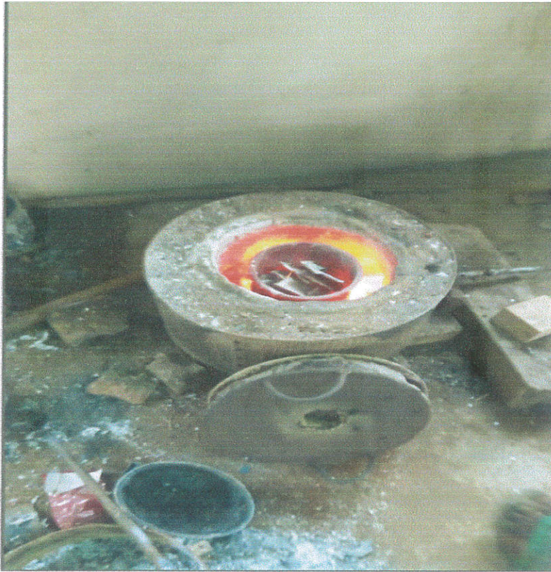
Figure 3.5: Charging of Aluminum into the blast furnace
