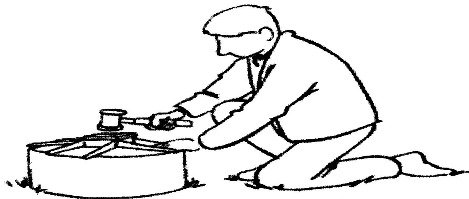
Fig. 3.5: Impact-Absorbing Hammer to Insert the Infiltration Ring
