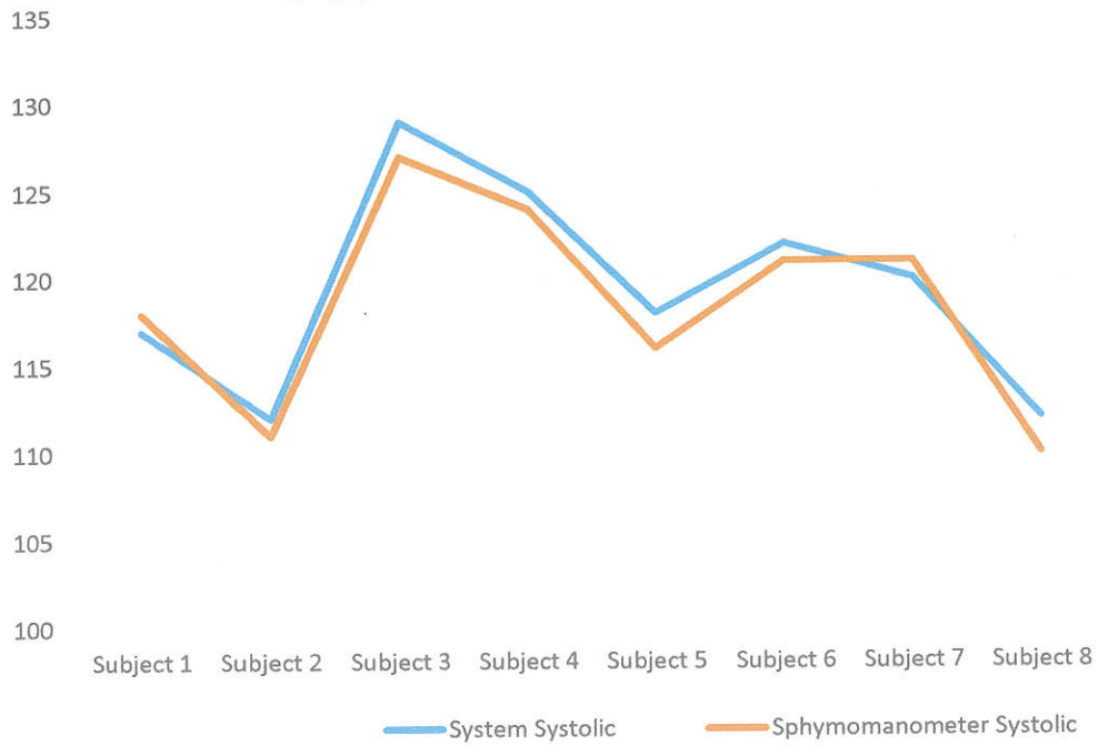
Figure 4.3: Comparison of Systolic Pressure in women from Designed System and Manual Sphygmomanometer
