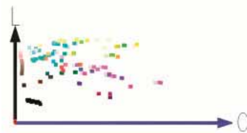
Figure 8. Arrangement of GretagMacbeth SG test target colours as a 2D projection of gamuts on L-C axes of LCH colour space after converting from RGB to CMY with Relative Colorimetric rendering intent and ACE CMM (when BPC is not activated colours are presented darker)
