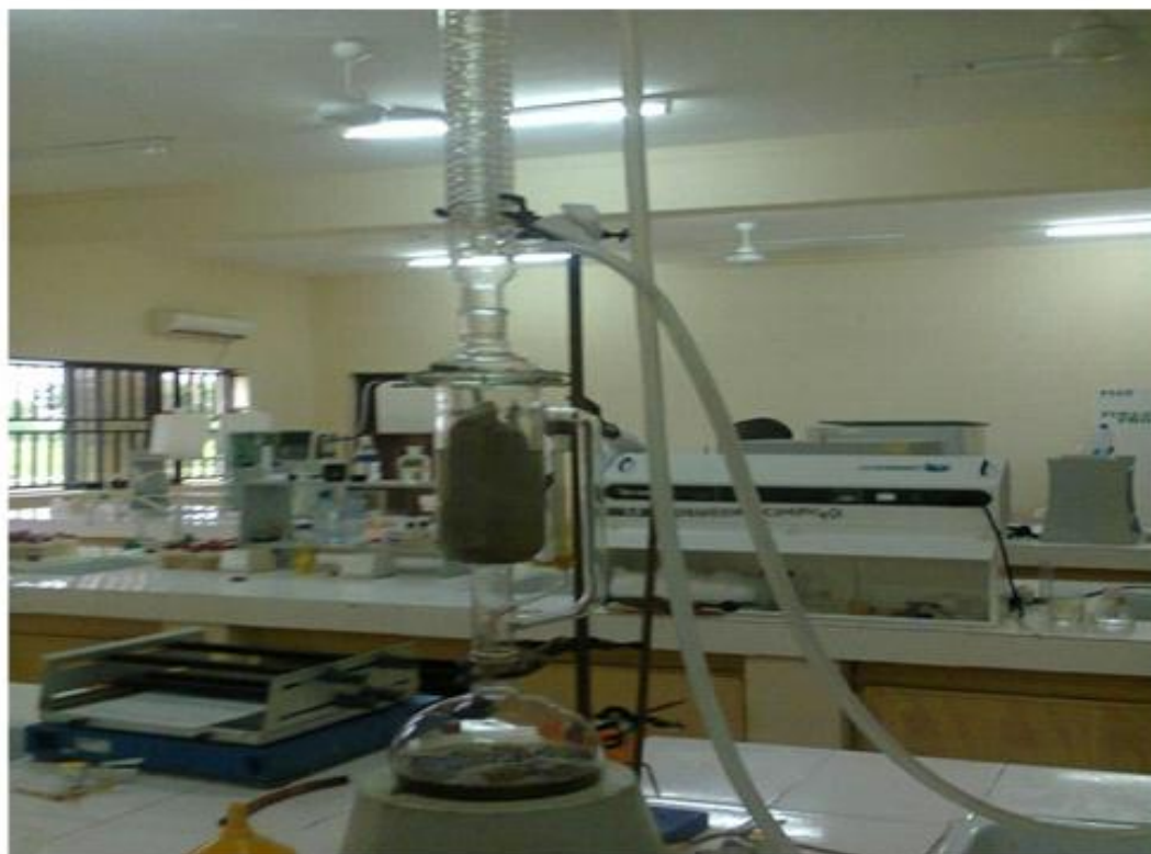
Figure 1. Soxhlet extraction set-up.
