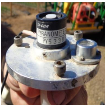
Plate 3. Pictorial view of Pyranometer used.
