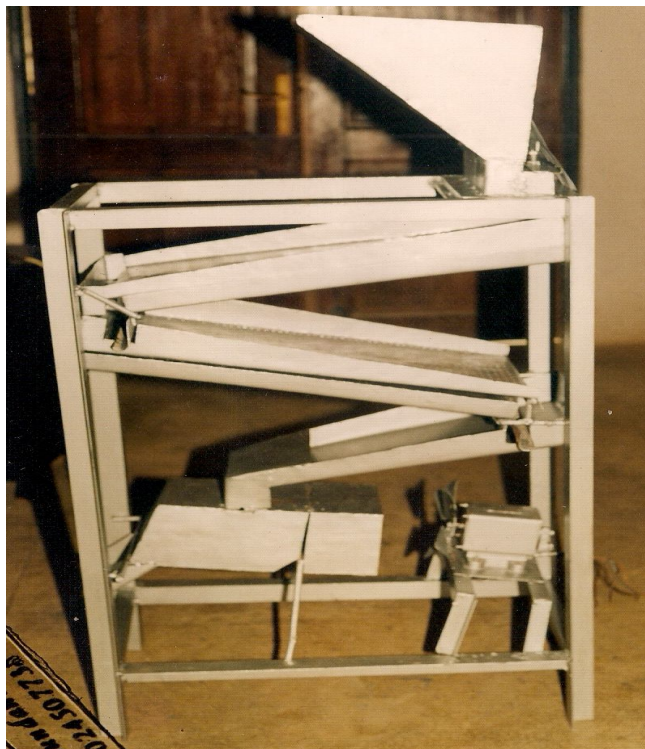
Fig. 3: General view of the rice de-stoning machine
