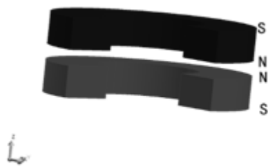
Figure 8: Homopolar permanent magnetic suspension ring pair
