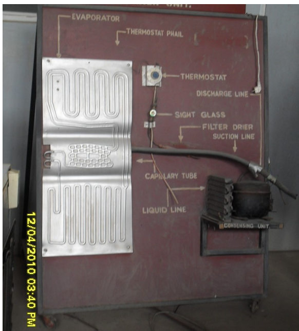
Fig. 3: General view of the experimental apparatus for demonstrating vapour compression refrigeration system
