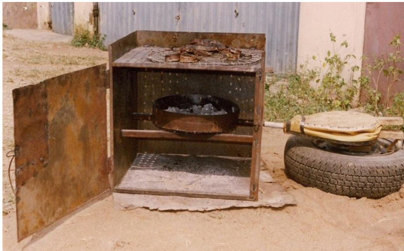
Fig. 1: Locally developed smoking kiln
