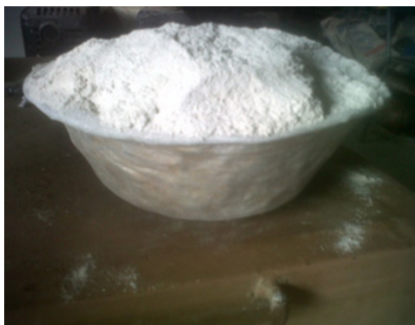
Figure 1. Roofing sheet waste (milled)
